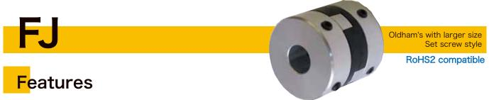
•Combination of aluminum hubs and a polyacetal slider to handle shaft diameters up to  $\phi$ 38 •High-precision slider groove for light press-fitting and zero backlash, enabling servo operation •Sliders can also be made of chemical-resistant or heat-resistant materials
